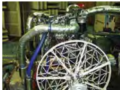
Using an 84-channel sector wheel array, beamforming and SONAH measurements were carried out in a hemi-anechoic chamber on both engine A (left) and engine B (right)
