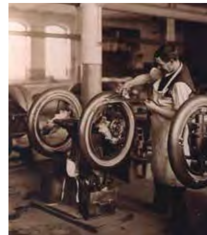
Tyre assembly at the factory in Hannover-Vahrenwald, 1921
