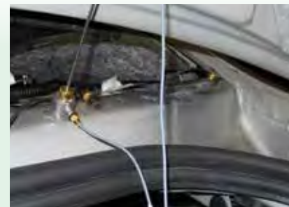
A force transducer and Type 4524-B accelerometers were mounted onto the car's rear deck to measure the FRFs
