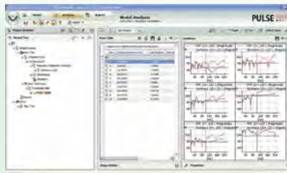
Comparing measured to synthesised FRFs using PULSE Reflex Modal Analysis
