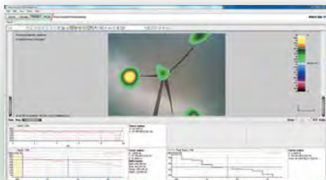
Result of sound intensity mapping from a beamforming measurement
