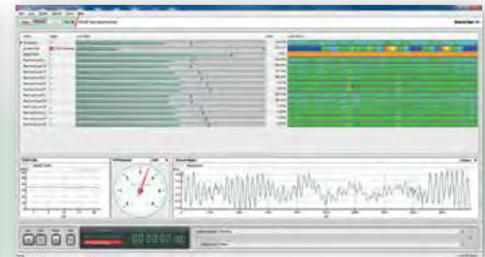
PULSE Time Data Recorder with a level meter indicating overload occurrences and coloured level history keeping track of optimal dynamic range selection
