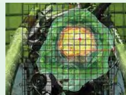
Mapping various metrics using beamforming. From top to bottom – stationary loudness, roughness, and combined metrics.
