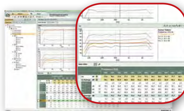
Typical building acoustics project using PULSE Reflex Building Acoustics Type 8780. Data are presented graphically and numerically with detailed quality indications using the smiley system on Type 2250/2270 hand-held analyzers.
