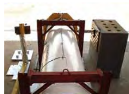
Launcher in support structure before firing test. During the launcher firing test, Brüel & Kjær Type 4956 microphones, Type 2670 preamplifiers, and a PULSE data acquisition system are used to obtain noise data.
