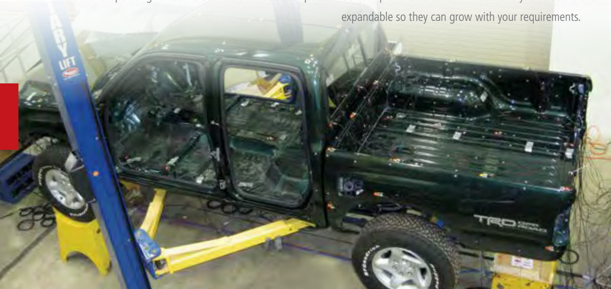
PULSE Modal Test Consultant seamlessly handles multiple shaker testing, providing accurate and reliable FRF data sets for the modal parameter extraction process
