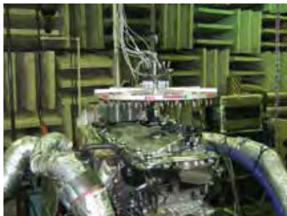
Using an 84-channel sector wheel array, beamforming and SONAH measurements were carried out in a hemi-anechoic chamber on both engine A (left) and engine B (right)
