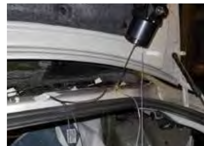
Mini-shaker Type 4810 used to excite the rear deck of the car to determine the stiffness of the structure
