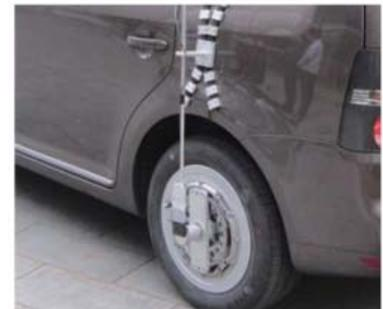
M4113 & M4115 - Wheel loadcell measure 6 axis loads of a wheel in a vehicle. M4113 fits 13" to 20" wheels, and M4115 fits 16" to 22" wheels. The slip ring 41150-RING-00 transmits the signal from the wheel loadcell to a data acquisition system via a small flexible cable
