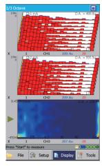
Supports continuous measurements and shows the results on waterfall or intensity plots
