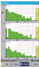
Display VC (Vibration Criteria) curves on 1/3 octave spectrums for quick evaluation of floor vibration.
