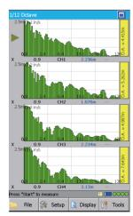
Real-time four channel measurements of Octave, 1/3 Octave and 1/12 Octave spectrums
