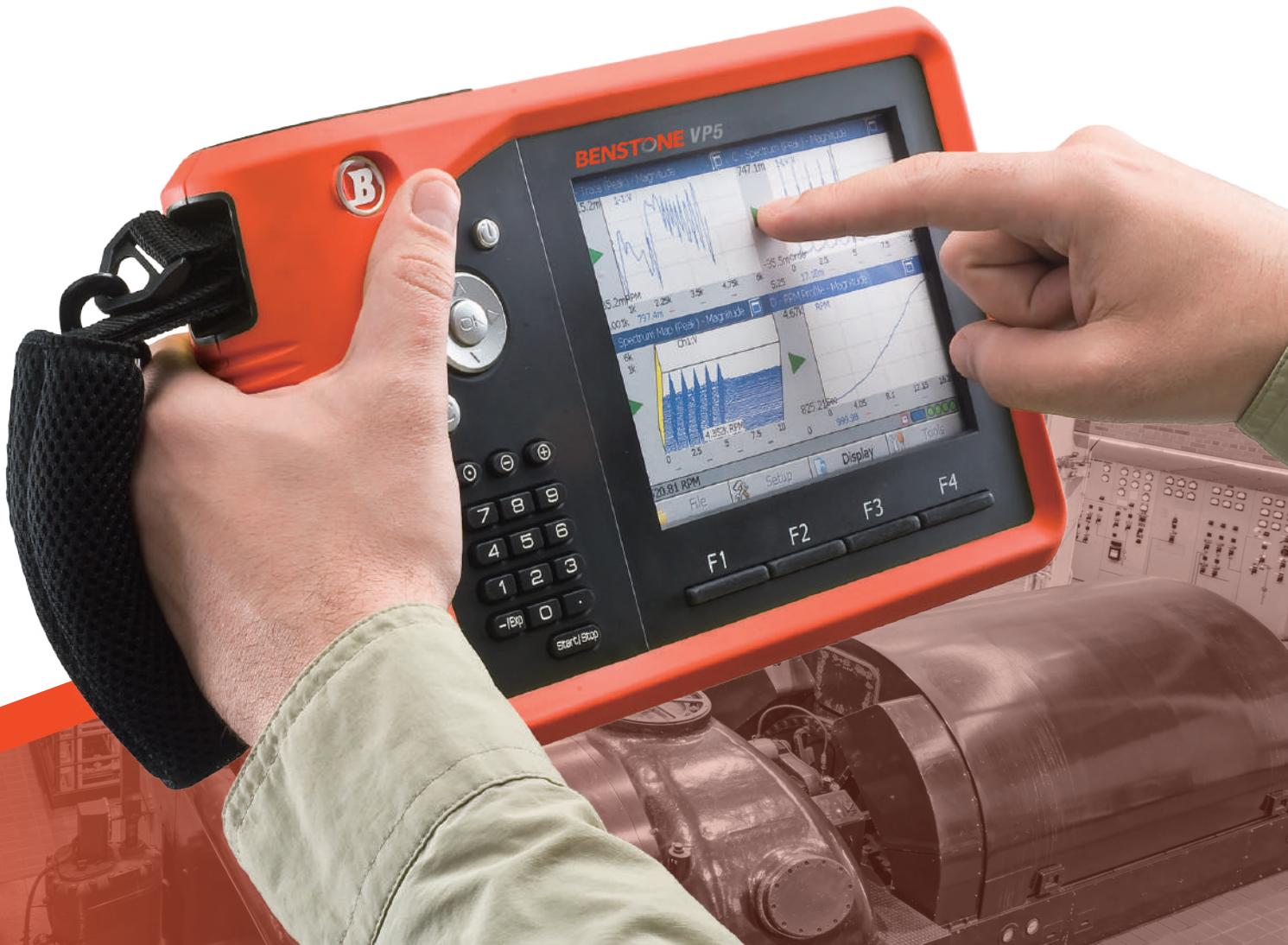
Measure cross channel functions, such as FRF and cross power spectrum, which are required by ODS testing
