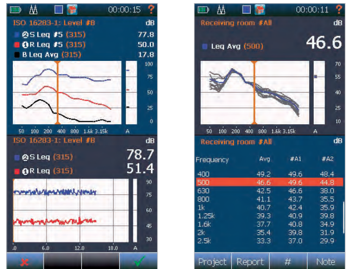
Split screen display (left) with Source, Receiving and Background levels in the upper level versus frequency (L/f) graph. The lower graph is a level versus time presentation of the Source and Receiving room based on the cursor position from the L/f graph. Alternatively, all microphone positions and the average values are displayed together (right).
