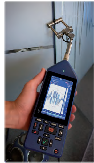
Sound Intensity probe used for noise source localisation
