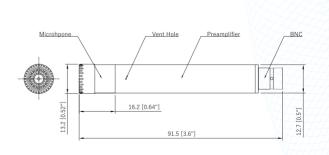
Fig.2 CRY361-S02 Microphone Set Drawings
