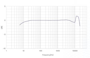
Fig.1 CRY361-S02 Microphone Set Typical Frequency Response
